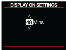
Use Up and Down buttons to change the LCD display on time. Press ENTER button to apply the changes. The default value is 10 mins (0 mins is "always on").
