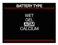
Use Up and Down buttons to choose your battery type which is marked on the battery case. Press ENTER button to apply the changes. The default type is AGM
