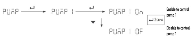
Figure 33 Water Pump Enable/Disable setting
