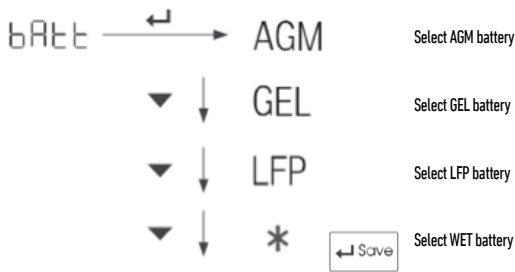
Figure 30 Battery Type setting
