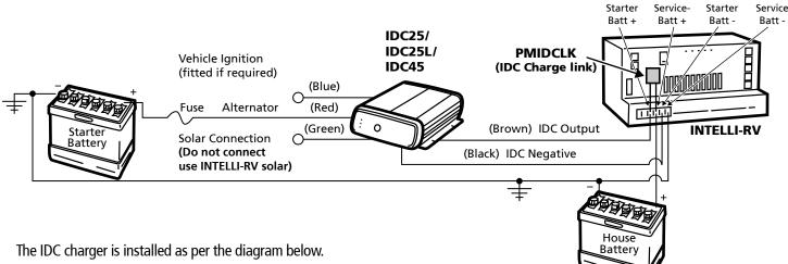
Note: Cables for IDC Alternator, Negative and Output should use 8B&S cable.
