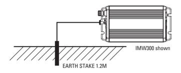
• External Earthing Mobile Applications – Connect an earth wire (Preferably solid Green or Green with Yellow stripe) from the external earth connection (Chassis GND) on the rear of the inverter to the chassis of the vehicle or ground wires in a boat.
