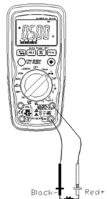
**NOTE:** A "good" diode will read low in one direction and high in the other direction when the probes are reversed (or vice versa). A defective diode will have the same reading in both directions or read between 100 to 3.0V in both directions.
