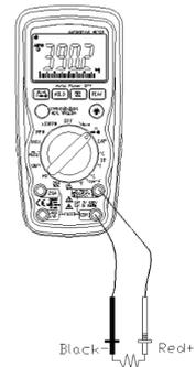
**NOTE:** Accurate measurement is not possible if external or residual voltage is present.
