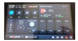
3. Go to the bottom of the menu selection the left, tap the blank space 3 times and enter password 1000.
