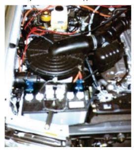
5. Reconnect the negative battery terminal to the main starter battery or install the desired Dual Battery System. Before closing the bonnet make sure the battery and tray do not hit the bonnet.
