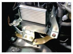
8. Bolt lower bracket on terminal box and bolt into position.
