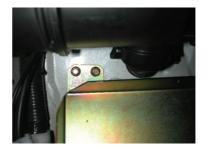
8. Push through 2 x M6 bolts through the holes and the wheel arch then support plate on the underside of the wheel arch. Tighten M6 nuts.
