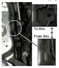
4. Unbolt junction of earth wires from inner guard, discard bolt.
