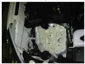
3. Unclip wiring loom and bolt in supplied right angle bracket using 1 x M6 bolt and nut. Hole created after unclipping loom clip.
