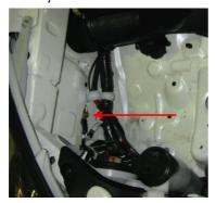
5. Fit the tray in position using 3 x M6 counter sunk bolts into captive nuts.
