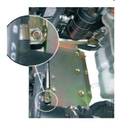
8. Fit battery onto the tray. Install J bolts and lay the Special Top Mount over the battery and J bolts. The top mount will line up with one of the bolts from the side guard. Remove this bolt and tighten the bolt using the spaces provided to the Special Top Mount and the side guard. Tighten the wing nuts on J Bolts and Special Top Mount.
