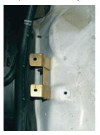
5. Lay the battery tray into position lining up the holes with the Special Tray Mounting Bracket.
