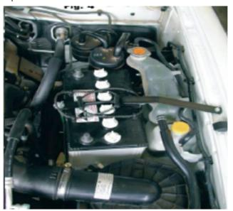
9. Reconnect the negative battery terminal to the main starter battery or install the desired Dual Battery System. Before closing the bonnet make sure the battery, tray and J bolts do not hit the bonnet.
