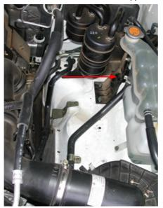
3. Remove bolt from bracket holding overflow bottle hose from inner guard.
