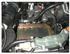
6. Bolt the tray into positon using the counter sunk bolts. Use the two captive nuts and one existing hole in the inner guard. Use the existing hole, bolt washer and nut provided.
