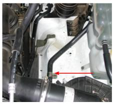
4. Fit Special Tray Mounting Bracket to inner guard. Use 2 x M6 bolts in to the captive nuts on the inner guard.
