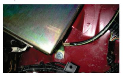
9. Place Auxiliary battery in rear tray towards the firewall.
