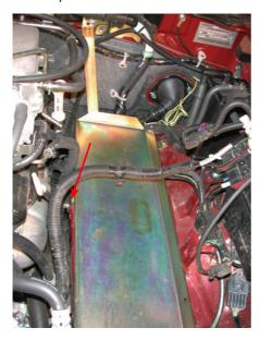
7. Use the M8 short bolt to bolt rear arm of the tray to the bracket of the firewall.
