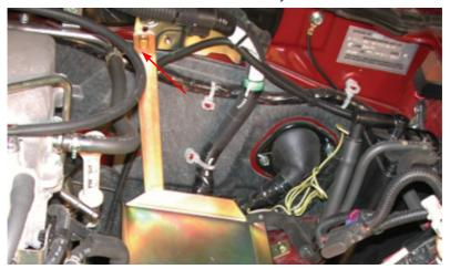
8. Using the 2 x M6 (Hex) bolts, bolt into remaining support holes, ensuring M6 body washers and nuts under guards. Existing holes may need enlarging, realign earth lead to provide room.
