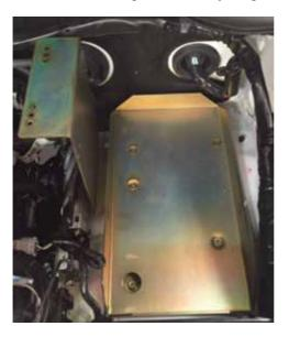
3. Place tray in position placing spacer washer underneath front hole in tray closest to guard. Without tightening, screw M6 counter sunk bolt to captive nut.
