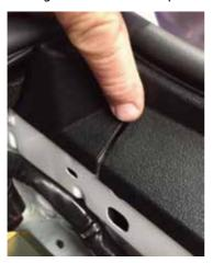
8. Using top mount Anchor Bracket mark hole centre and drill two 9mm holes. Using a Rivet Nut gun install 2 x Nutserts (Supplied) in to top of guard. Insert M6 bolts and secure anchor bracket to top of guard.
