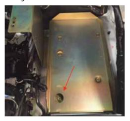
6. Drill hole through guard at the rear of the tray closest to the guard and secure with M6 countersunk bolt, nut and body washer.
