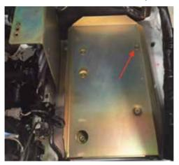
7. Free mould on top of guard and locate the top mount anchor bracket through existing slot in mould. Mark position on guard. Remove moulding.
