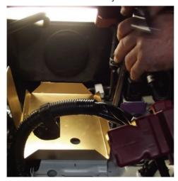
11. Fit M6 bolt through hole at front of tray into captive nut.
