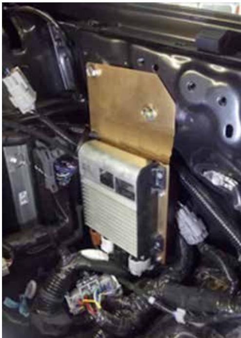
5. Remove factory accessory fuse box from its bracket from the inner guard. The fuse box may be redundant when the dual battery system is completed. For the time being cable tie to the wiring harness between battery and intercooler.
