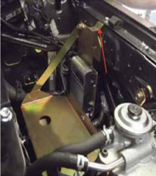
8. Reconnect plugs to "Injector Driver" computers and bolt brackets in inner guard captive nuts, using 1 x M8 short bolt at front and 1 x M8 long bolt at rear (leave loose, as they need to be removed as tray arm fits over computer mount plate).
