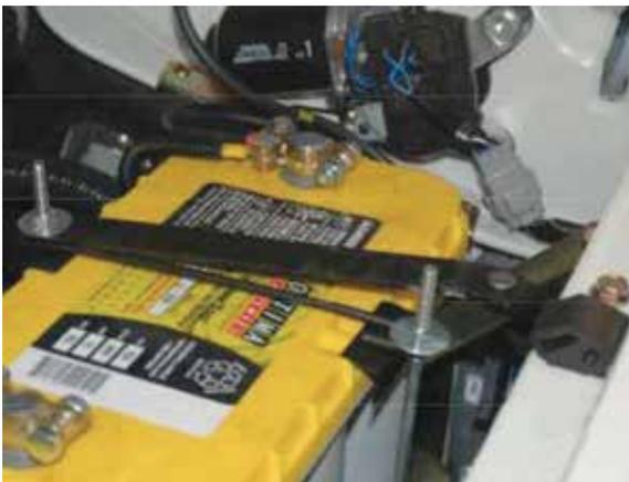
14. Reconnect the negative battery terminal to the main starter battery. Before closing the bonnet make sure the battery and tray does not hit the bonnet. You may now wish to fit your desired Dual Battery System.
