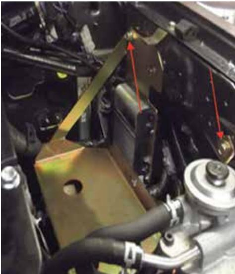
11. The fitter needs to ensure there is sufficient clearance between tray, wiring looms, fuel lines and air conditioning pipes. E.g. Ensure windscreen washer tube is not kinked or restricted when moving computers.
