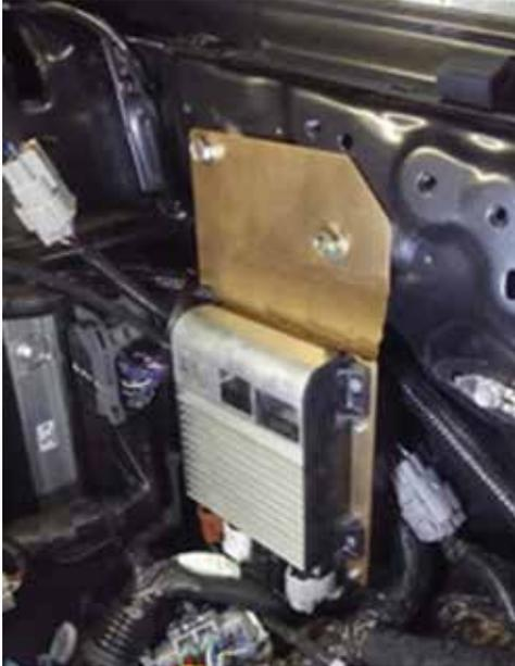
10. Place tray into position and bolt in upper arms with 1 x M8 short bolt for front arm of tray and 1 x M8 long bolt for rear arm of tray, the bolt needs to go through rear arm and the computer plate bolting to the inner guard captive nuts. The tray can be flexed slightly forward or back to aid clearance.
